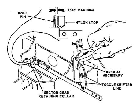
Bend the vertical members of the Toggle Shifter Link so that the Roll Pin in the Sector Gear Retaining Collar will at no time be more than 1/32 inch from the side of the nylon Stop, as the Transfer Motor cycles.
