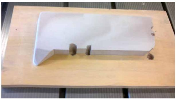
After working the panel 'in" You make a box around the worked in panel. Make shure in every direction you have a good draft angle (at least 0,5 degrees), and take care for a good loosing . Then you pour a 2 component resin in .
