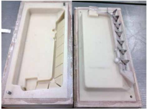
Place the two mold parts together , and pour in some 2 component resin in the mold through the holes created by the iron pins.
